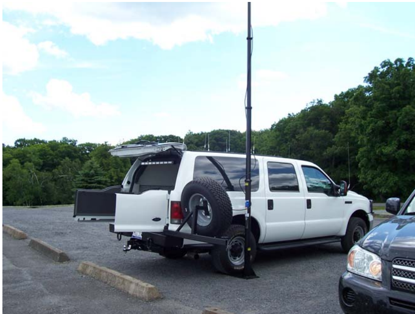
RAMER vehicle in action with the 35-foot collapsible antenna mast at the Helderberg Cell Site, Thatcher Park, NY.
