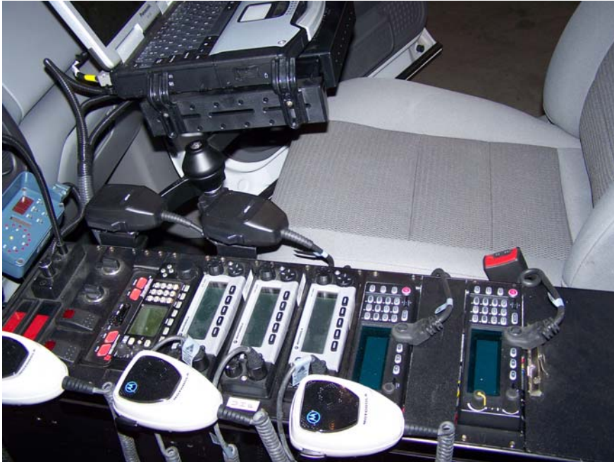
Center console showing legacy radios (front) and OpenSky radios (rear)
