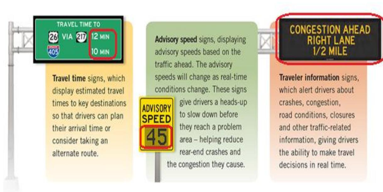
The ATM system was designed as a **long-term solution**. It consumes data from a variety of sources including field VOS (Volume Occupancy Speed) devices that gather information about vehicle traffic, as well as weather and highway traveler condition databases.
