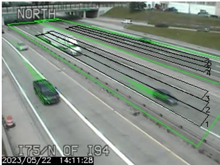
Figure 2: AID Lane Monitoring and Detection
