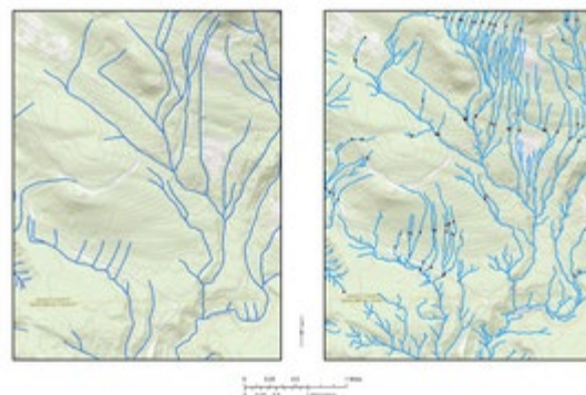
Figure 1: Graphic showing the improved alignment possible in the 3D Hydrography Program by deriving hydrography data from high-quality lidar elevation data
